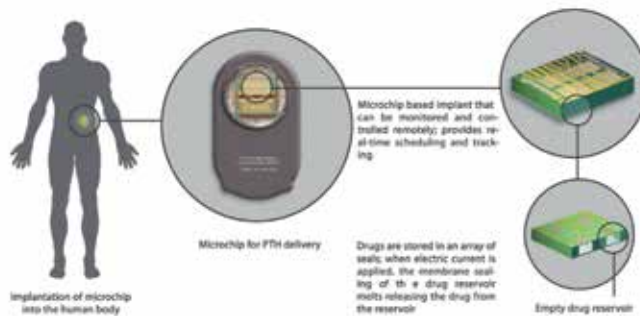
Figure 6. An implantable microchip for releasing parathyroid hormone fragments (1-34) (PTH(1-34)) (Fenu et al., 2012).
